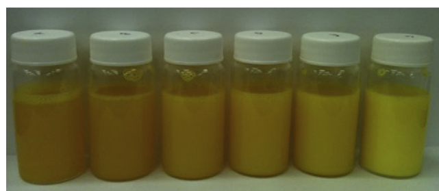
Fig. 4. Appearance of aqueous PS-FBMS nanoparticles (67 mg/mL) of increasing size (35 ± 5 nm (left) to 87 ± 12 nm (right)).
